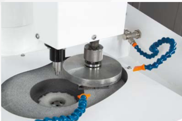
Prepolishing of large raw samples.
