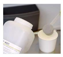
that, in addition to the high reproducibility of the embedding, offers a high level of safety at the workplace due to its easy handling. Furthermore, the product does not emit any harmful substances and can therefore be used without an extractor hood – ideal for routine mountings e.g. during production.
