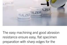
resistance ensure easy, flat specimen preparation with sharp edges for the vast majority of materials. The cleaning of the specimen with water-based agents is very quick and simple.
