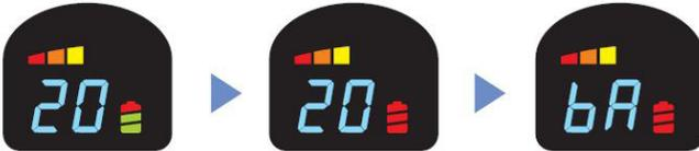
1. If battery level indicator is all green, it shows fully charged battery, and all change to the red, it shows the time to charge.
