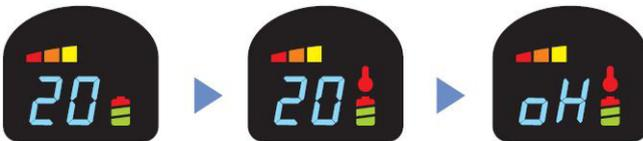
1. If the temperature of the power LED climbs up above the setting temperature, overheat warning indicator will be on.
