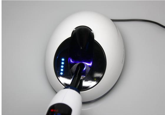
Put the end of the light guide at the middle of the oval shaped indicator and irradiate light. You can check and see the optical output instantly. Please note there can be occurred an accidental error depends on the location and angle of the light guide.
